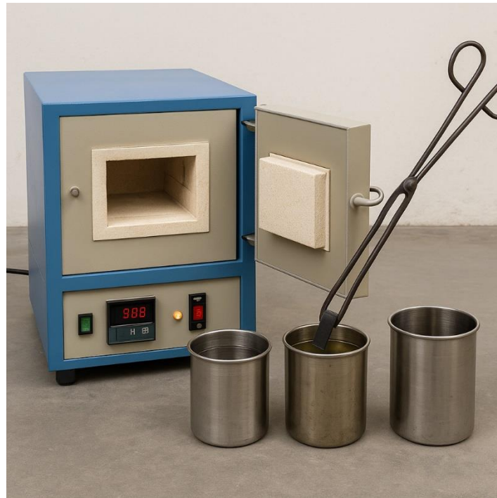
Figure 1. Laboratory furnace and quenching setup used in the experiment.
