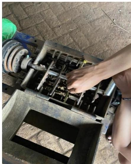
**Gambar 2.** Proses Pengaturan Jarak Clearance
