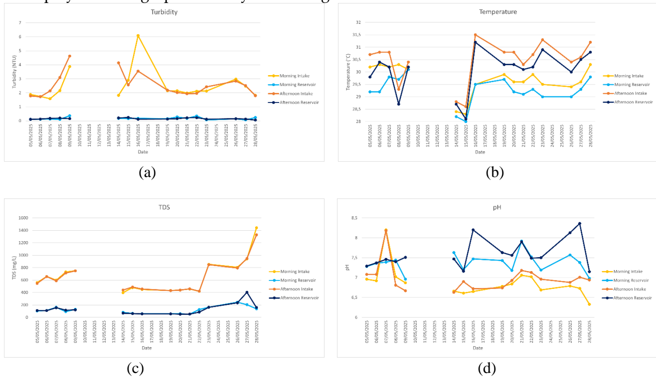
Figure 3. Graphs of Raw Water and Treated Water Test Results Based on (a) Turbidity, (b) Temperature, (c) TDS, and (d) pH in May 2025
