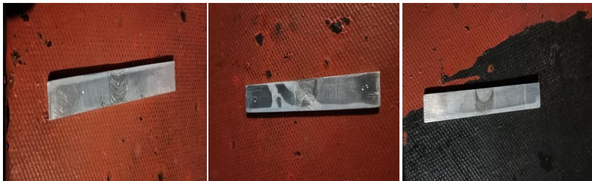
Gambar 5. Hasil uji kekerasan : (a) specimen 1 (b) specimen 2 (c) specimen 3
