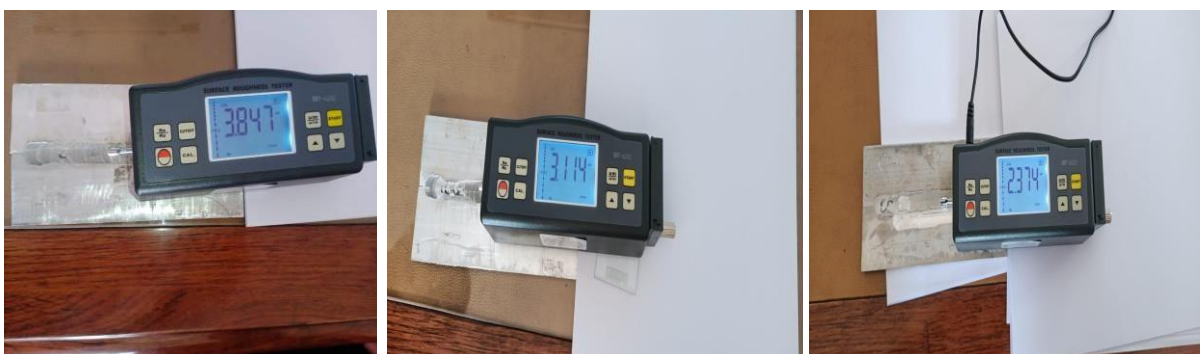
Gambar 7. Hasil uji kekasaran : (a) specimen 1 (b) specimen 2 (c) specimen 3
