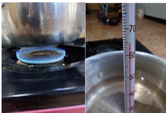
Figure 3. Measurement of water temperature after boiling with LPG fire
