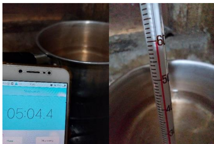
Figure 2. Measurement of water temperature after boiling with fire from biogas
